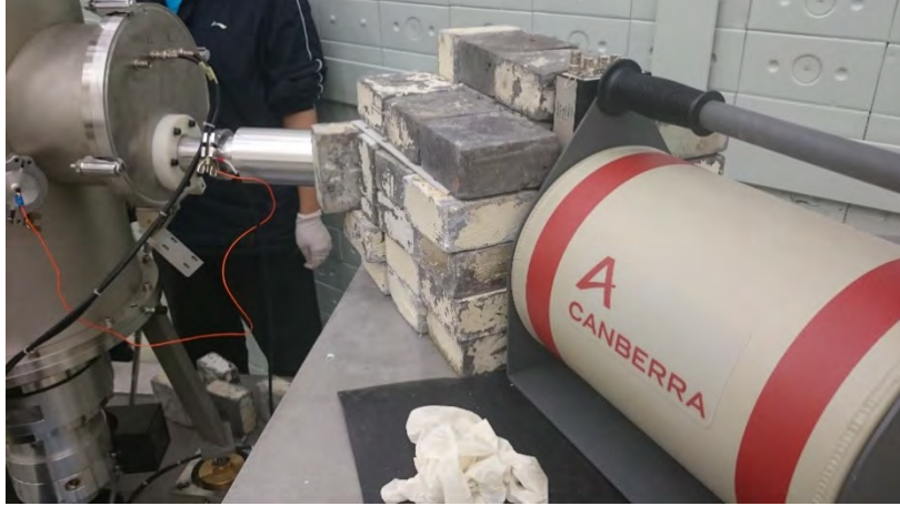
Figure 7. HPGe detector 100% relative efficiency placed at 55^\circ at the reaction chamber.
