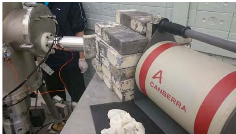
Figure 5. HPGe detector 100% relative efficiency placed at 55^\circ at the reaction chamber.
