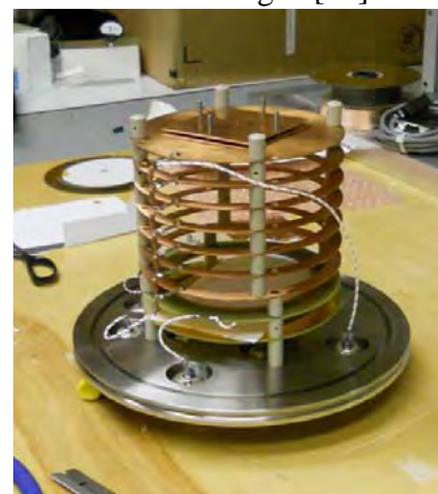
Figure 21. Picture of AstroBox1 from pre-experiment setup. Beam enters perpendicular on cylinder axis.
